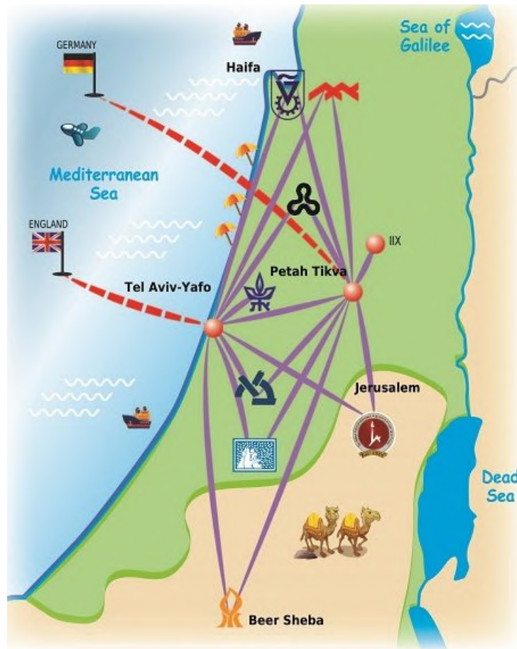
Figure 1.2: The communications fiber network connecting Israel’s main universities [47]. The red dashed line represents two international links to the European GEANT network and through these to the American research network Internet2.
